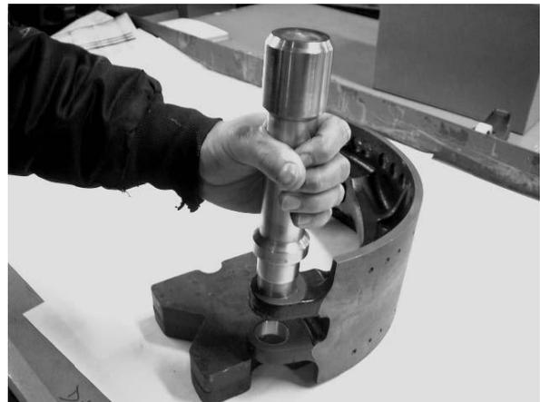
Figure 10- Bushing removal/installation tool
