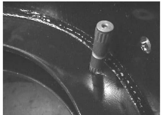
Figure 11 – Installation of brake shoe return spring pin
