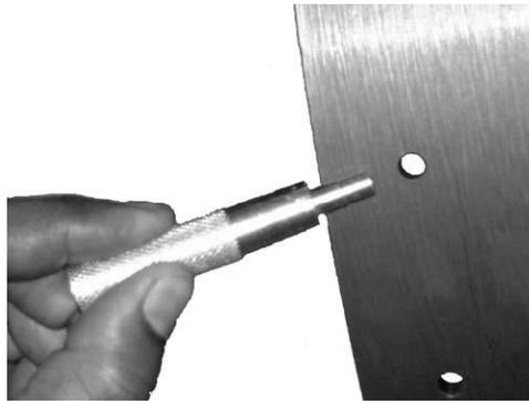
Figure 7 – Bolt/rievet hole measurement
