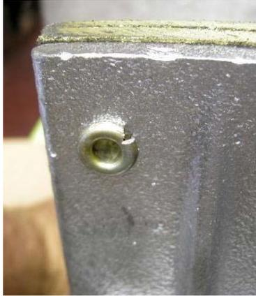
**Figure 15a - “Slice of pie” cracks or cracks that extends into solid or “hole” portion of rivet shank**
