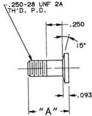
Figure 2 - Cast Plus brake bolt
