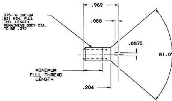
Figure 1 - W type brake bolt
