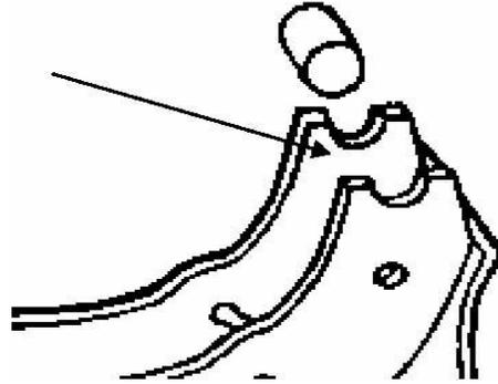
Figure 9 - Roller seat inspection
