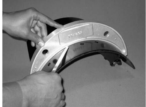
Figure 5 – Table arc measurement
