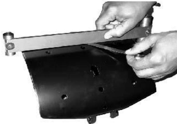
Figure 3 – Measurement of shoe flatness
