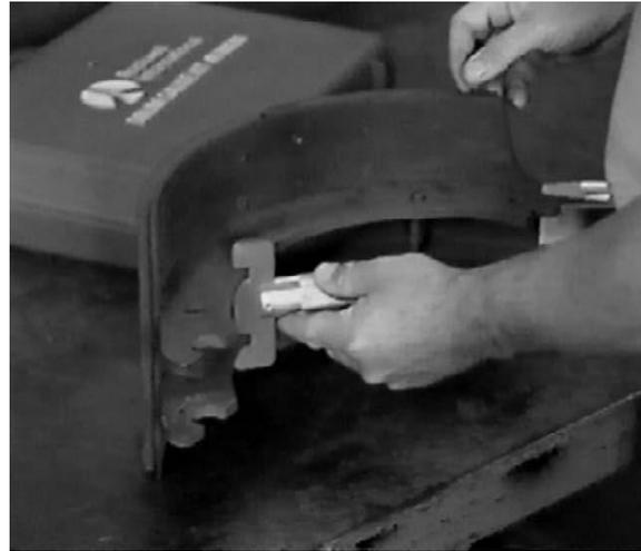
Figure 4 - Using a go/no-go gauge
