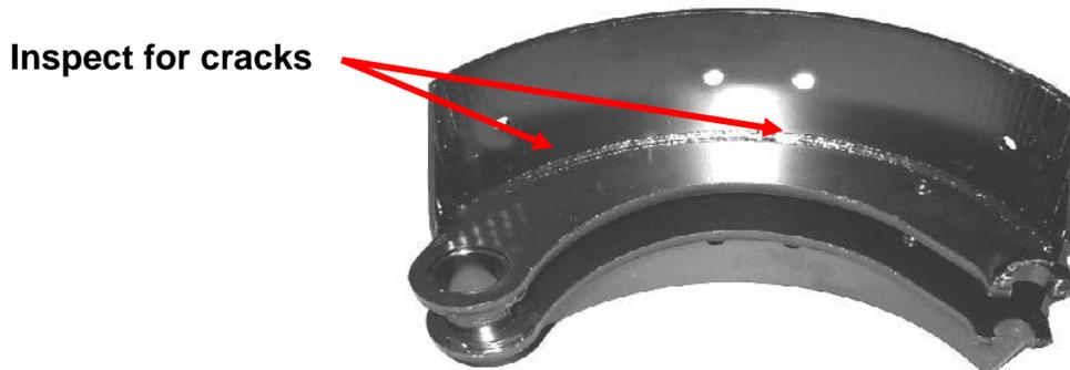
Figure 8 – Shoe weld Inspection
