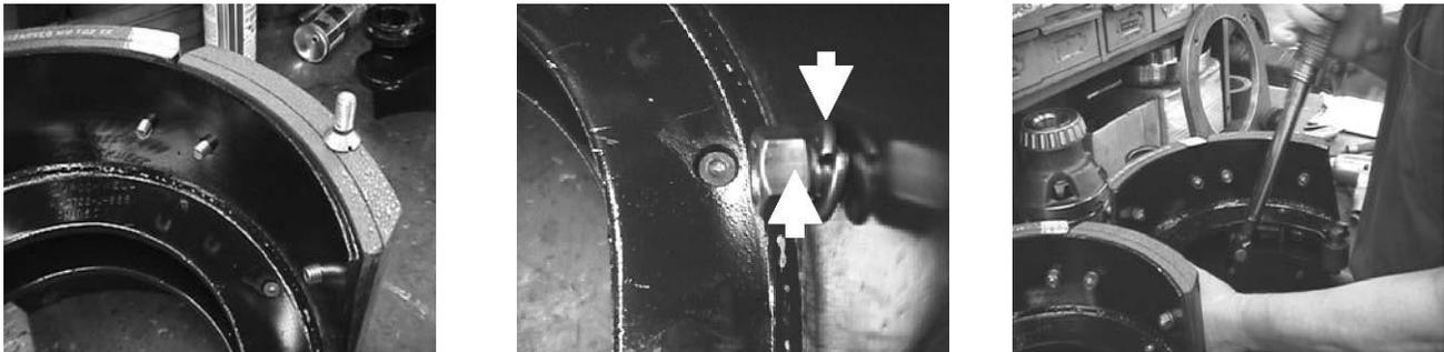
**Figure 16 – Block fastener installation**
