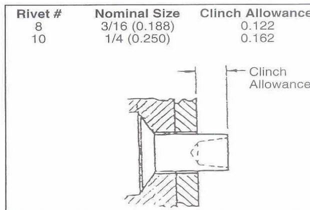
**Figure 13– Rivet Length Calculation**
