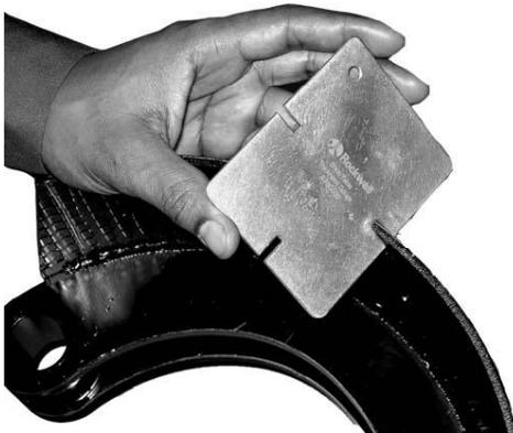
Figure 6 - Measuring stamped steel shoe table thickness
