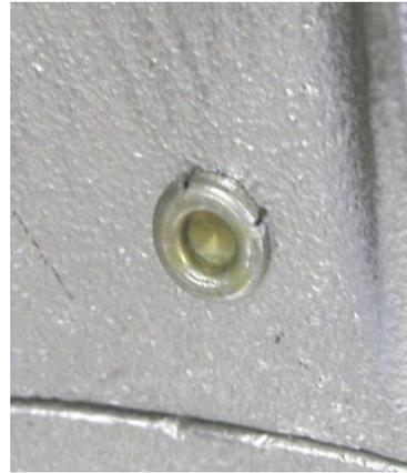
**Figure 15b - Multiple hairline Cracks**
