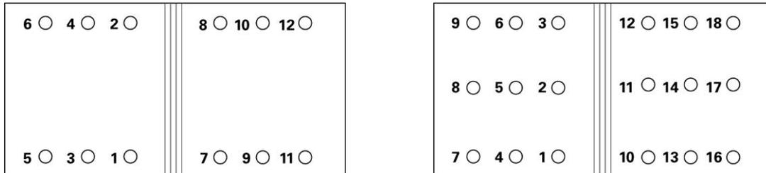
**Figure 14 –Typical fastener attachment sequence**
